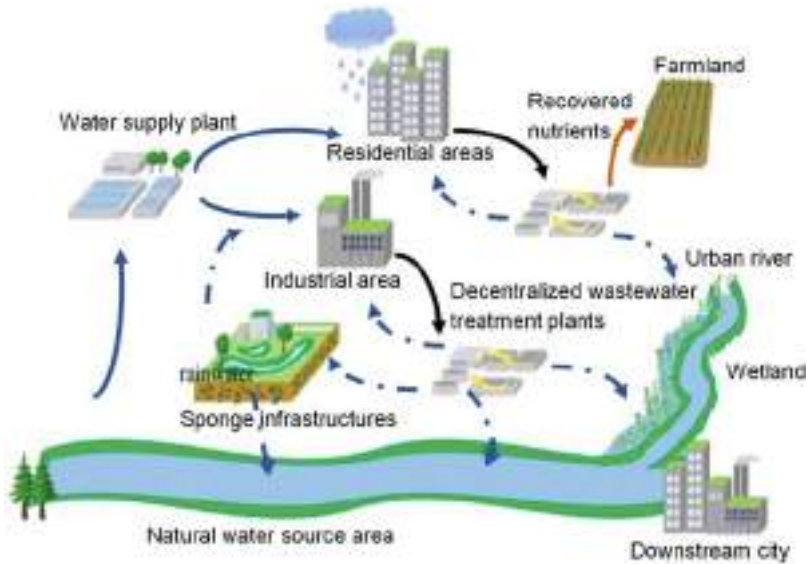
Figure 3.4 Depiction of urban water system 3.0 (figure by authors; blue, grey, brown and yellow arrows represent water flow, wastewater flow, resource supply, and energy supply, respectively).
