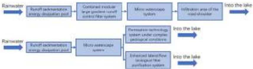
Figure 13.6 Technology framework of rainwater treatment for the demonstrative project (figure by authors).
