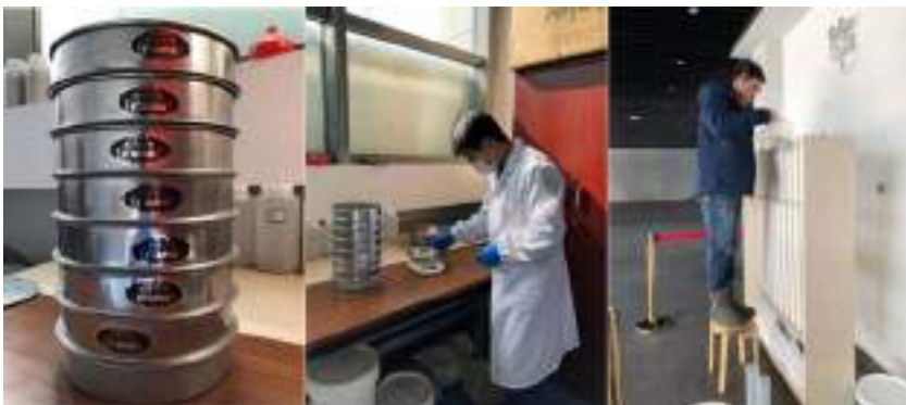
Figure 5.7 Laboratory experiments for selection of media (left – particle size distribution test; right – infiltration tests).
