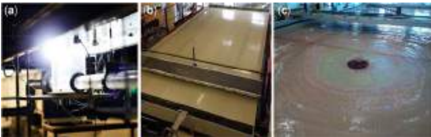
Figure 9.2 Example of experimental urban flood models with sub-surface interaction ( Rubinato 2015 ). (a) View of the scaled drainage system of the sub/surface experimental facility at the University of Sheffield; (b) Birdseye view of the urban floodplain of the sub/surface experimental facility at the University of Sheffield and (c) experimental simulation of sewer overflow. ©MatteoRubinato.
