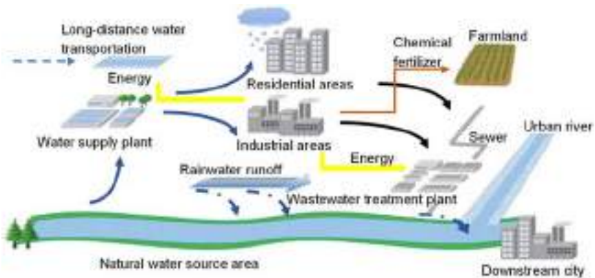
Figure 3.2 Depiction of urban water system 2.0 (figure by authors; the blue, grey, brown and yellow arrows represent water flow, wastewater flow, resource supply, and energy supply, respectively).
