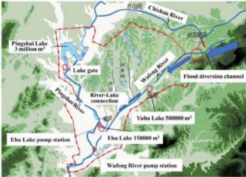
Figure 11.12 Layout of the large-scale drainage system for Pingxiang City (adapted from Pingxiang Sponge City Pilot Construction Summary Report (unpublished) 2018).
