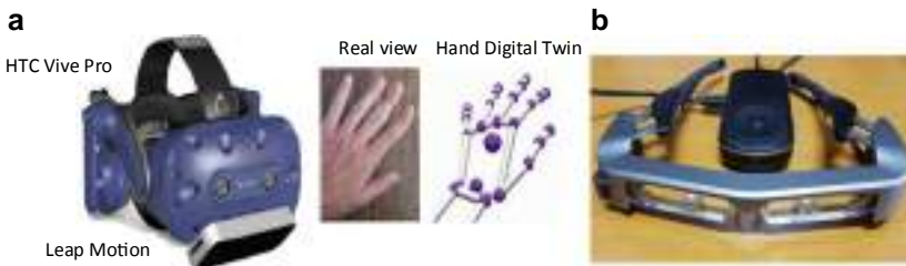
Fig. 2.18 Assisted assembly (a) Virtual Reality device HTC Vive Pro and Leap Motion, (b) Augmented Reality device Epson Moverio BT350
