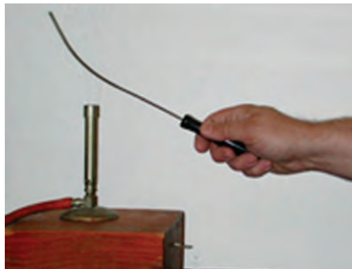
Sumber: www.physics.upenn.edu Gambar 4.6 Saat dipanaskan, bimetal melengkung.
